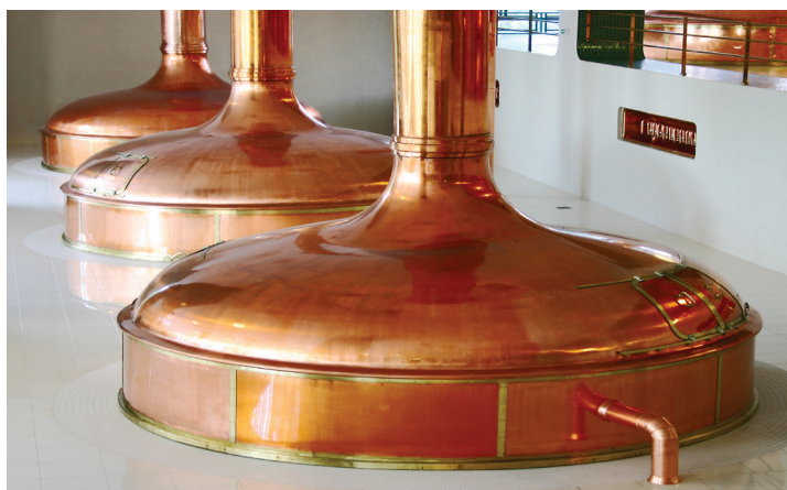
Polyclar Brewbrite wort clarifier and beer stabilizer is added to the kettle 5-15 minutes before the end of the boil.
